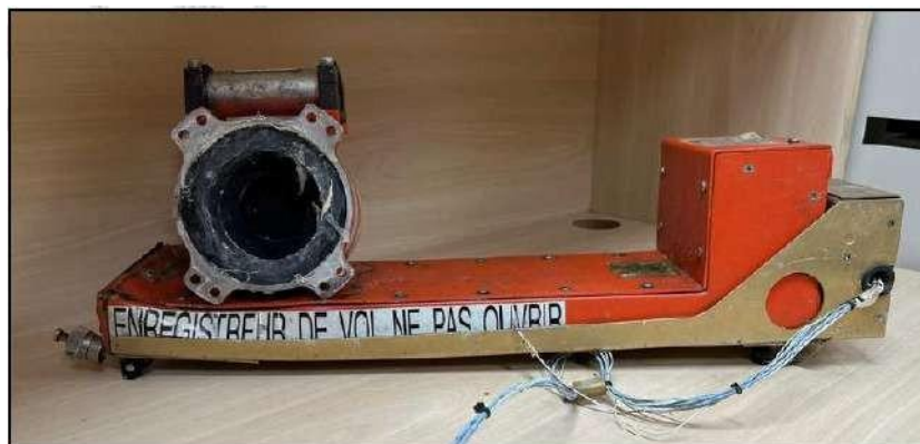
Figura 29 - Flight Data Recorder instalado na aeronave PS-VPB.
