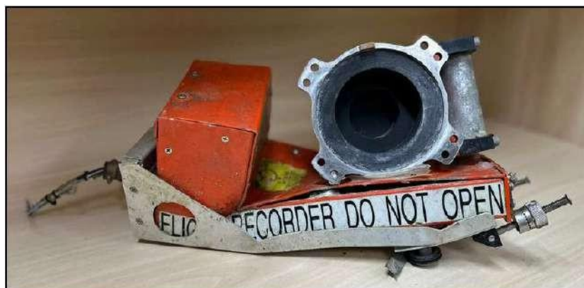
Figura 30 - Cockpit Voice Recorder instalado na aeronave PS-VPB.
