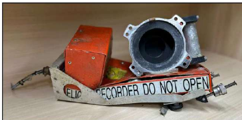
Figura 30 - Cockpit Voice Recorder instalado na aeronave PS-VPB.
