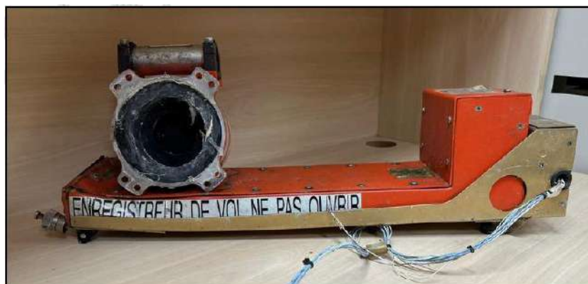
Figura 29 - Flight Data Recorder instalado na aeronave PS-VPB.
