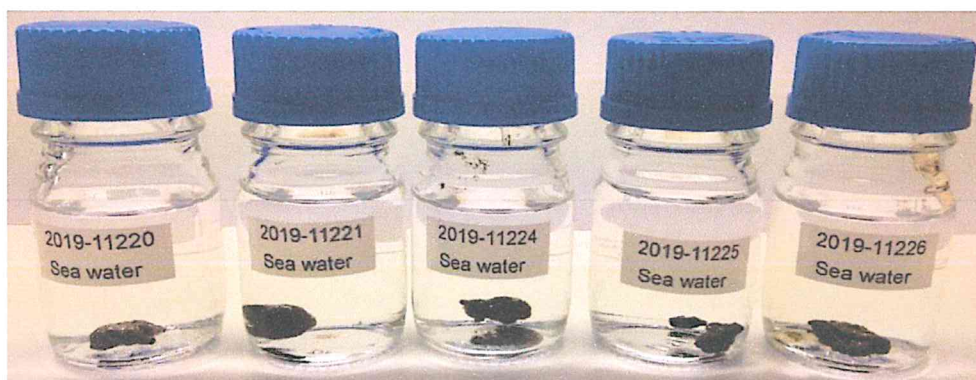
Figure 4.1 "Sinking test" of the spill samples in seawater.
